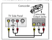
Locate the A/V output jacks on the camcorder. They are usually found on the side or back of the camcorder.
